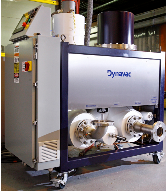
Figure 1. Typical gaseous nitrogen thermal conditioning unit (TCU). This 170 m 3 /hour TCU can provide up to 10 kPa of head pressure over a temperature range of -180 °C to 150 °C.
