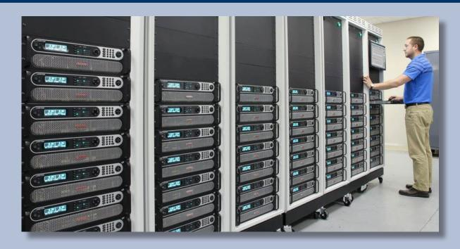
Dynavac's Auxiliary Thermal Control Systems (ATCS) adds auxiliary heating and power to flight hardware during test periods. Our flexible design platform enables customization of power channels and DC power output ranges to best suit your testing criteria.
